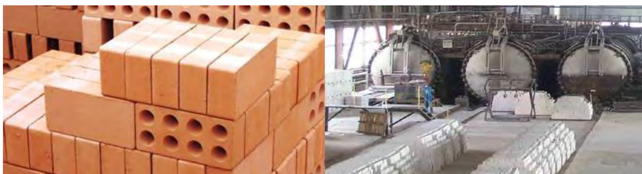
Fig. 2. Ceramic Bricks (left) and Silicate Products (right) on the Basis of Coal Mining Wastes
